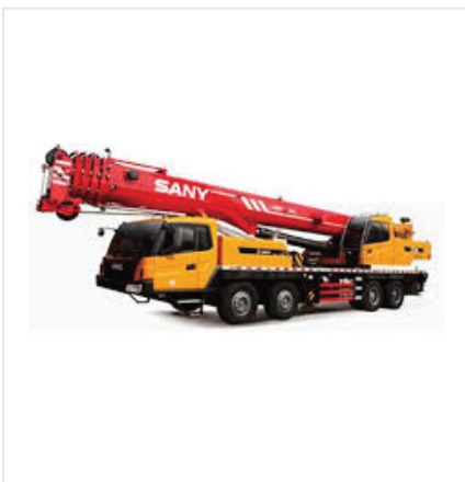
Truck Crane 100 Ton 60 Mtrs
