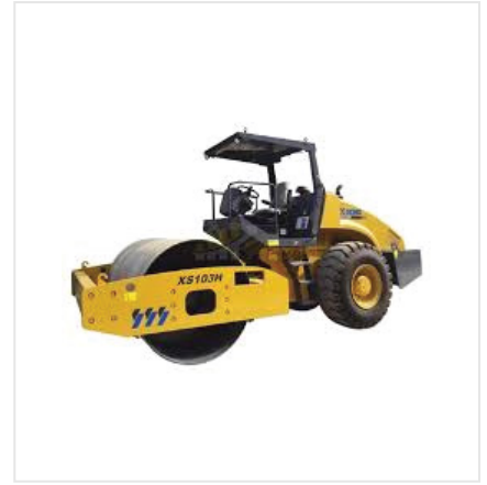
Roller Compactor 10 Ton
