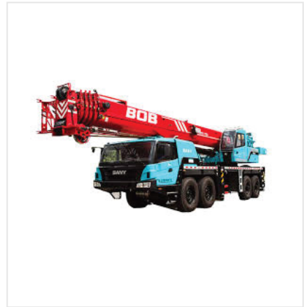
Truck Crane 100 Ton 52 Mtrs
